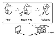
Once the T-4555 is ready for use, you'll need to tune into an AM radio station and adjust the position of the AM antenna to achieve the best possible reception.
